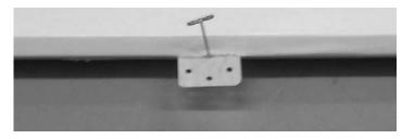
2. Install the e-z hinges in the stab using a pin in the center of each to make sure they stay aligned.
