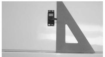
4. Install a control horn on the servo and center the servo with the arm paralle to the hinge line. Locate the position for the control horn by laying a 90 degree triangle down. Keeping the bottom of the triangle parallel to the hinge line and the top even with the outer servo arm hole.
