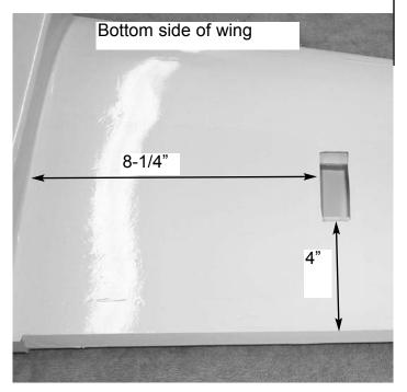
2. Locate the servo hole in the wing and remove the covering with a #11 blade.
