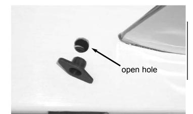
4. Using your #11 blade, open the hole on both sides of the fuselage. Install the mounts in both sides using the 2mm screws supplied. There is an access hole in the bottom of the fuselage for installing the plate on the inside.
