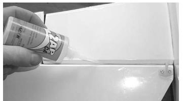
3.Install the elevators on the hinges and with the elevators pushed tightly against the stab, remove the pins. Using thin CA, glue each hinge in place by applying two to three drops on each hinge. Have the elevators deflected to full up when gluing the bottom side of the hinges and deflected to full down when gluing the top side of the hinges. This will insure that you can get full throw later.
