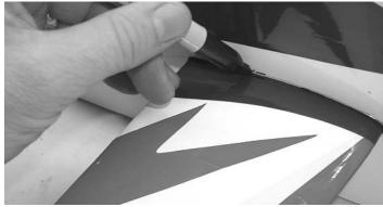
4. When satisfied with the alignment, use a dryerase marker to draw a line on side of the stab, top and bottom where it meets the fuselage. Remove stab from opening.
