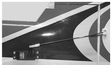
3. Locate the 2-56 x 10" pushrod and thread a clevis on the end.(Don't forget the silicone keeper) Install a servo arm on the servo and center the servo. The servo arm should be positioned pointing up parallel to the rudder hinge line. Mark the location for the bend and make a 90 degree bend. Cut off at 3/8" and install in the servo arm using the swing in nylon keeper to retain it. The hole in the servo arm will need to be drilled to a 5/64".
