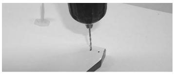
1. While the epoxy dries on the stab, mount the control horns on the elevators. Align on the inside edge of elevator on the bottom side, with the holes on the horn aligned over the hinge line. Use a square to check alignment of holes over hinge line, this is important to maintain even throw on both elevators. Use a long drill, piece of wire, or pencil to mark the holes through the control horn. Remove the horn and drill the holes using a 5/64" drill.
