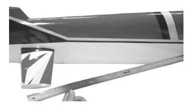
3. With the stab centered, measure from one tip to the back of the wing cut out. Move stab until this figure is the same on both sides.
