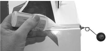
5. using pins to center the hinges as was done with the elevators, install the rudder. Deflect to full throw and glue the hinges in place using thin CA.
