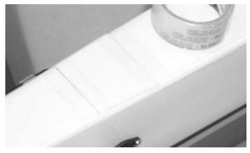
6. you can mount the hatch cover on the bottom of the fuselage using clear tape or screws (not included)
