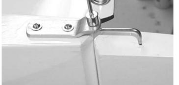
3. Place tailwheel on the bottom of the fuselage so that the wire is flush with the back of the fuselage and centered on the bottom.
