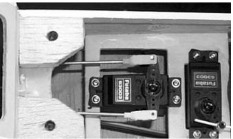
7. Center the elevator servo in the tray and mount the servo using the hardware supplied with the radio.
