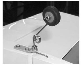
4. Mark the location of the tail wheel wire on the rudder and drill a 5/64" hole into the rudder to accept the tail wheel wire.
