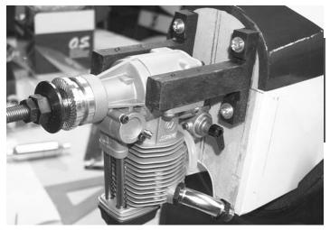
5. Align the motor on the firewall. Center the engine on the off center vertical line and the horizontal line. Drill holes on the marks using a 3/16" drill. Insert the blind nuts into the rear of the fire wall and tighten using washers and lock washer (use thread lock).
