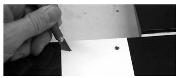
6. Using the #11 blade, remove the covering over the rear wing bolt holes on the top of the wing.
