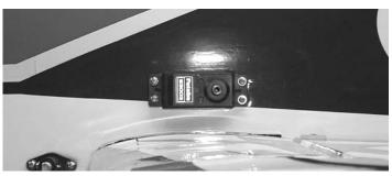
2. Install the rudder servo using the hardware supplied with the radio. You will need an 18" extension added to the servo lead.
