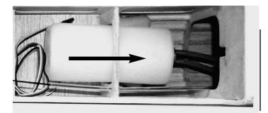
3. Install the tank in the fuselage in the notches provided in the bulkhead, and hold in place with foam(not provided). Attach the fuel lines(not provided) to the three metal lines and route through the hole in the firewall and to your engine. If you are using an engine without a pump or pressure system you will probably have to mount the tank in the nose of the plane.
