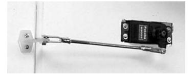
6. Screw a 4-40 nut and metal clevis on each end of the 4-40 pushrod. Adjust the length of the pushrod till the aileron is level.
