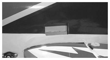
1. Remove the covering over the rudder servo cutout with your #11 blade. It is just above the elevator bell crank hole on the right side of the plane.
