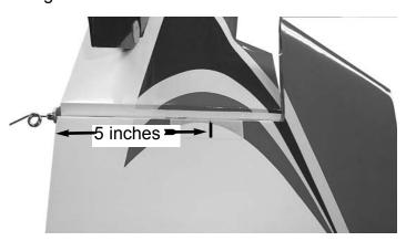
6. Locate the rudder horn 5" from the bottom edge of the rudder on the left side. Mark the holes and drill using 5/64" drill as was done with the elevator. Mount the horn using the 2-56 x 1" bolts and nylon plate. Twist the control horn so that it is facing the rudder servo hole.
