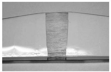
5. Using the #11 blade, remove the covering on the top and bottom of the stab between the lines. Cut about 1/8" inside the lines so that there is no exposed wood when glued in place. Be careful to cut only the covering and not into the wood of the stab as this would weaken the stab.
