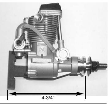
Note: The distance that is shown is for using a Carl Goldberg spinner. If you are going to use a different spinner, the front of the cowl needs to be 4-5/8" from the firewall.
