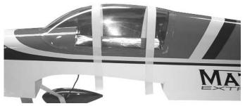
2. Position canopy and check fit. When happy with fit glue in place with ZAP canopy glue. Use masking tape to hold in place till glue dries.
