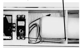
7. Mount the throttle servo in the servo tray ahead of rudder servo. Position the servo so that the servo arm is on the same side as the throttle pushrod. This may vary depending on the engine used. Glue the nylon sleeve to the bulkhead to prevent flexing of the rod. Install another e-z connector on your servo arm and attach to the throttle pushrod.
