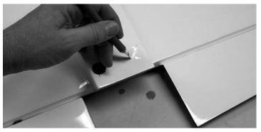
7. Turn the wing over and remove the covering over the wing bolt holes. Slide the front wing dowels in to the holes in the fuselage saddle. Push down on the rear of the wing till it sits in the fuselage. Using two wing bolts and washers, screw the wing down to the fuselage.
