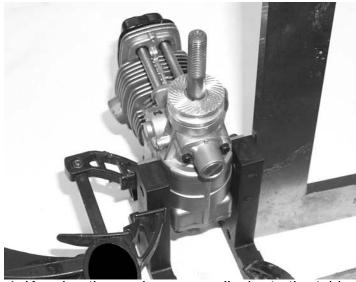
4. Keeping the engine perpendicular to the table top, clamp the other motor mount to the engine. Mark and drill the second motor mount then screw the mount to the engine.
