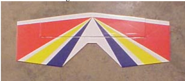
Horizontal Stabilizer, Elevator, and CA hinges
