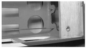
2. ☐ Insert one of the .072 x 27-1/4" threaded rods into the elevator pushrod tube.
