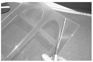
2. ☐ Using scissors, cut around the outside of the windows leaving a 1/8" flange around the edge.
