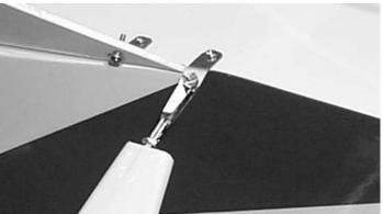
**4.** ☐ Hook the bottom of the strut to the aluminum bracket on the bottom of the fuselage.
