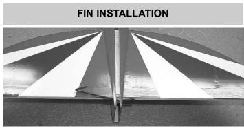
Insert the elevator joiner in through the space behind the stabilizer slot.
