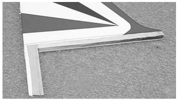
□ TAKING CARE NOT TO CUT INTO THE WOOD STRUCTURE UNDERNEATH, and working inside the drawn lines, carefully remove the covering where the fin mounts on the fuse and stab.
