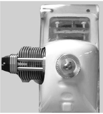
3.  $\square$  Keep the hole in the front of the cowl centered on the engine.
