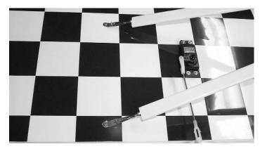
**5.**  $\square$  Attach the wing to the strut by screwing the clevises in & out to the straps.
