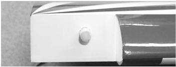
2. ☐ Using epoxy, mount the 5/16 x 1-3/4" dowels into the holes in the notch of the leading edge of the wing. Make sure to leave about 1/2" of dowel sticking out of the front of the wing. You may wish to slightly taper the exposed dowel ends for ease of insertion into the fuse holes.
