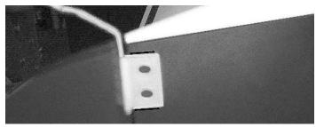
Mark where the tail wheel bracket meets the fuselage.
