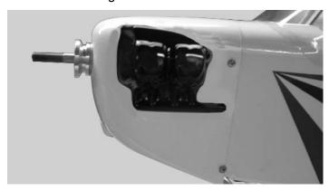
**4.** □ Screw the cowl to the fuselage using #2 x 5/16 screws.
