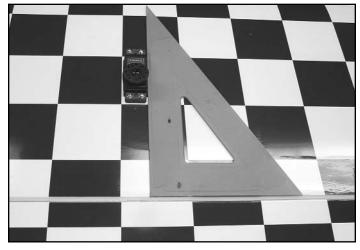
With the aileron servo in place, make a mark at a 90° degree angle to the trailing edge and in line with the side of the servo.
