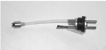
**4,** □ Install the 4mm silicone tube to the short brass tube and install the clunk to the other end of the silicone tube. This is the fuel pickup and must be free to "flop" around in the tank so it can pick up fuel in any attitude.
