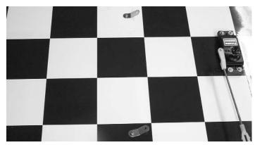
3. ☐ Using #2 x 3/8 sheet metal screw, mount the bracket so that it is pointing to the fuselage.
