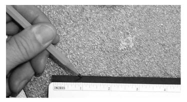
**1.**  $\square$  Mark 1" up from the bottom of the rudder.
