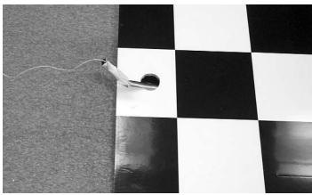
**IMPORTANT!** To ensure that any connections located inside the wing will not come loose, either when the wires are pulled, or during flying, always tape them securely together with electrical tape.
