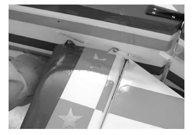
2. Locate the hole in the fuselage side and install the 2-56 pushrod into the pushrod tube already installed in the fuselage.
