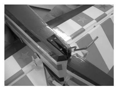
**6.**  $\Box$  Use the four #2 x 1/2" screws to mount the tail wheel bracket to the bottom of the fuselage.
