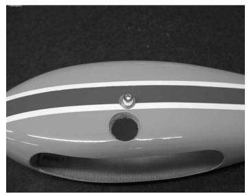
**4.** Install the blind nut in the wheel pant using the 4-40 bolt to pull it into the hole.
