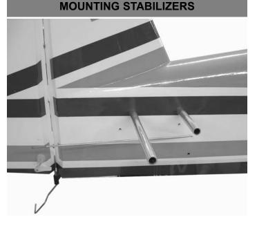
**1.** □ Insert the two aluminum tubes in the fuselage sides.
