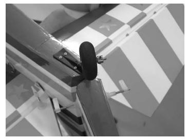
**7.**  $\Box$  Install the tail wheel using the wheel collar.
