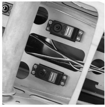
Install the two servos in the servo tray in the 4. rear most holes.
