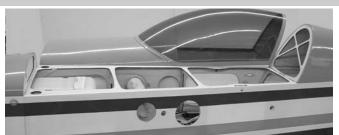
The top front half of the fuselage is a hatch. Remove the 4-40 socket head bolts on the side of the fuselage to disengage the hatch.
