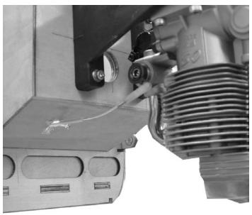
**3.**  $\Box$  Drill a hole(1/4") in the motor box that will give you the most direct access to the servo.
