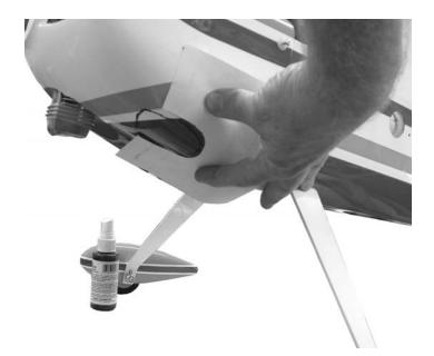
8. C Reinstall the cowl and transfer the hole location to the cowl.
