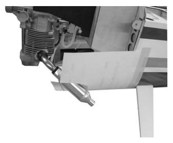
**7.** □ To locate the muffler exit, install the muffler, cut a piece of paper (Not Included) to fit around it leaving about 1/2" clearance and tape to the side of the fuselage.
