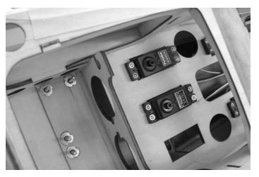
7. □ Install the rudder servo in the center slot of servo tray.
