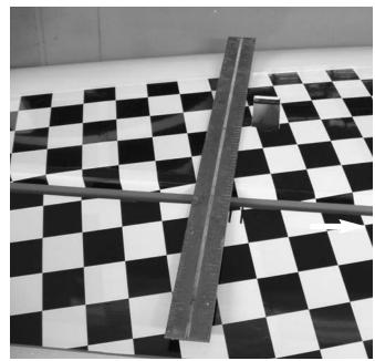
2. □ With the aileron servo in place, make a mark on the aileron at a 90° degree angle to the trailing edge and in line with the servo. Look for the control horn hard point under the covering. This is the location for the control horn.
