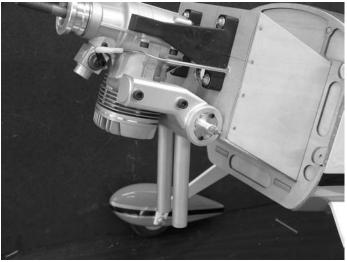
7. □ To locate the muffler exit, install the muffler, cut a piece of paper to fit around it leaving about 1/2" clearance and tape to the side of the fuselage.
