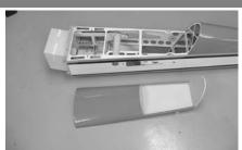
The top front half of the fuselage is a hatch. Remove the 4-40 socket head bolts on the side of the fuselage to disengage the hatch.
