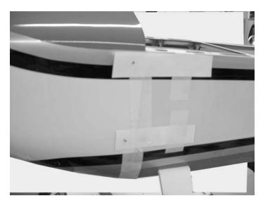
**3.** □ Mount the cowl in position and hold in place using masking tape.
