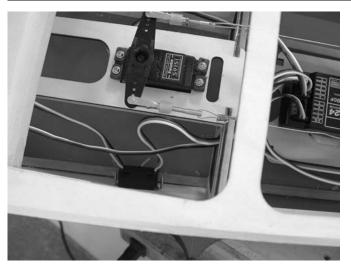
**1.** □ Switch mount positions are provided on both sides of the fuselage, either can be used.
