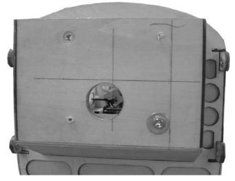
**4.** □ Using the 3mm mounting bolt and washer pull the blind nuts into the firewall.
