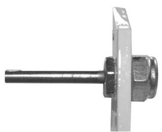
**3.**  $\Box$  Mount the axle to the landing gears.
