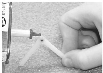
3. □ Place 1 drop of oil on each of the hinge joints at the center. This is to keep the hinges loose and prevent epoxy from sticking at the joint.
