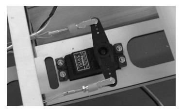
7. Connect the two clevises to the output arm on your servo.
