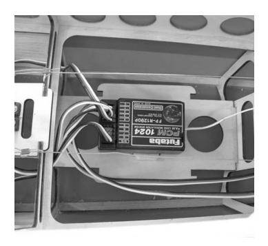
**2.**  $\Box$  A mount for the receiver is provided just behind the servo tray and under the rudder cables.
