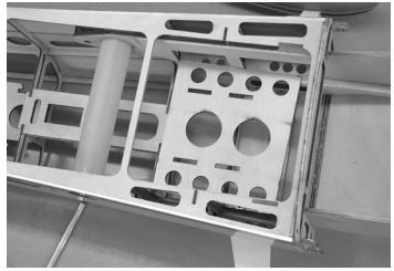
8. □ If you use a gas motor or motor with a pump, the tank floor can be installed in the rear most position which will put the tank closer to the CG.
