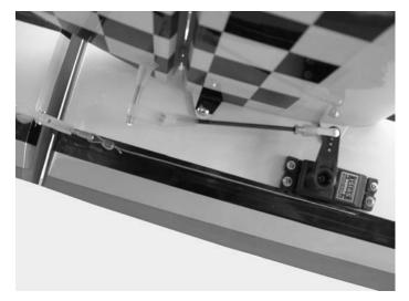
**4.** □ Thread the cables through the holes in the fuselage side located just under the elevator servo.
