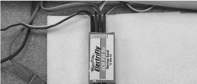
3.  Plug the elevator and rudder servos into your receiver.
