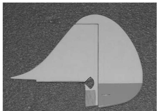
2.  Remove the covering off the bottom of the rudder hinge post.
