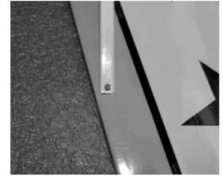
3.  Screw the wing strut to the bottom of the wing.
