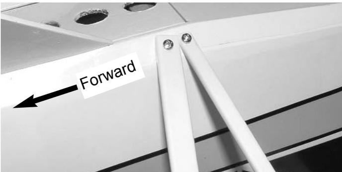
2.  Screw the wing struts to the fuselage using the #2 x 5/16 philip head screws.
