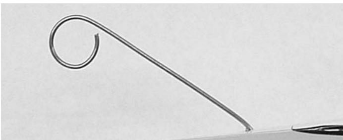
2.  Insert the tail skid wire into the bottom of the fuselage under the tail in the pre-drilled hole.
