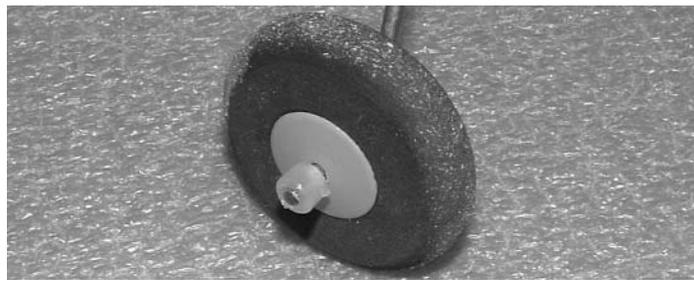
3.  Place the wheel onto the wire and hold it in place by inserting the Nylon retainer on the end.
