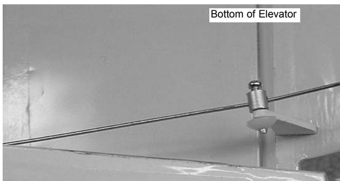
2.  Locate the slot in one side of the elevators near the center.
