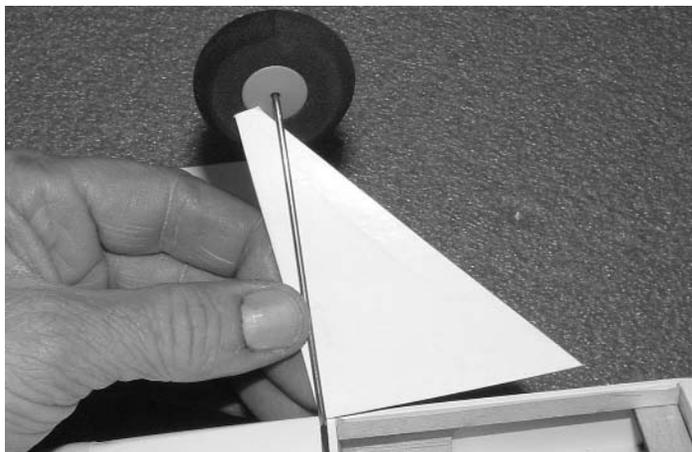
4.  Place the landing gear fairing on the fuselage.
