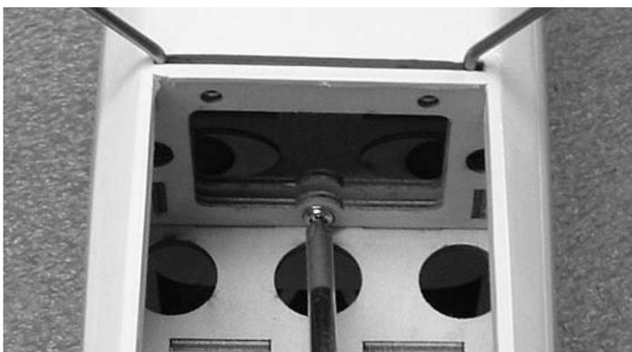
2.  Remove the hatch from the bottom of the fuselage
