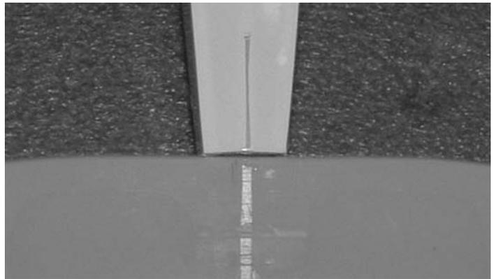
2.  Draw a center line 2" up from the stab on the fuselage
