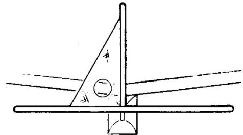
2. \* Insert the fin into the fuselage slot.
