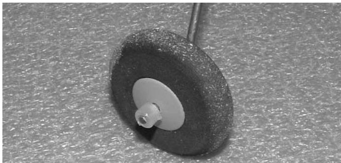
3. \* Place the wheel onto the wire and hold it in place by inserting the Nylon retainer on the end.
