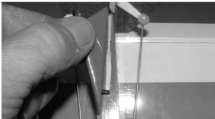
2. \* Insert the wire exiting the bottom of the tail skid into the hole in the bottom of the fuselage.
