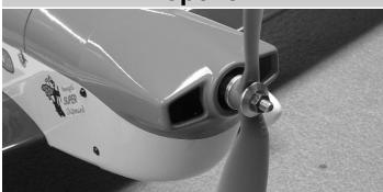
Install the prop adapter and your propeller at this time. We used a 9 x 4.7 APC prop for our motor, battery and speed control setup.
