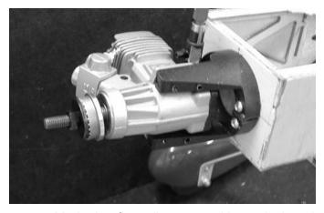
6. ☐ Mark the firewall center with vertical and horizontal lines. Offset the vertical line 1/8" to the left to compensate for the right thrust.
