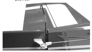
**5.** Repeat steps 2 through 4 for the rudder pushrod and control horn.
