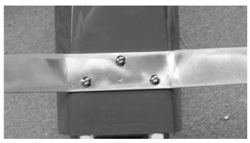
2. ☐ Mount the the main landing gear on to the bottom of the fuselage using the 4-40 x 1/2" bolts.
