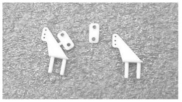
**2.**  $\square$  .Remove the back plate off the control horns.
