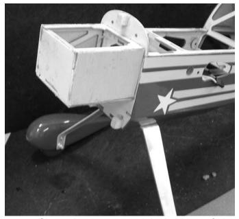
5. □ Sheet the bottom and both sides of the motor box with 1/16" plywood.
