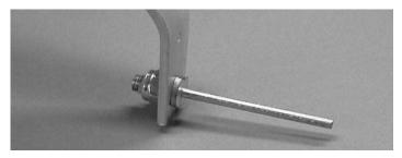
**2.** □ Install both axles on the landing gear.
