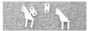
Cut the back plate off the side of the control horn.
