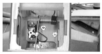
**10.** □ Glue the throttle servo in place and attach the throttle pushrod to the e-z connector.
