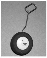
3.  $\square$  Place the wheel in the wire and insert the tubing on the end of the wire.
