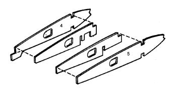
**6r.** With the rib notches pointing down, and the plywood reinforcement facing inward, place the reinforced tabbed rib at the #5 rib location.
