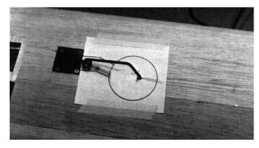
Mount the main retracts back into the wing and tape down the wheel well template included with this kit.
