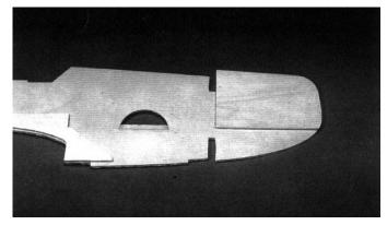
6a After gluing the fuselage doubler to each fuse side, glue the retract nose doubler to each side, using the front edge of the motor mount as a guide.
