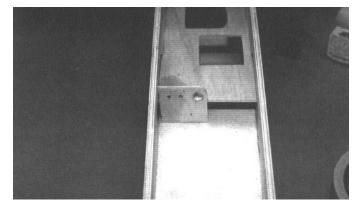
After making sure the servo tray is glued into position, glue the air-valve holder onto the end of the servo tray.
