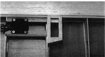
Trim the balsa servo cover, so that the edge reaches the center of the top of rib #5, leaving room to glue the bottom sheeting to the other half of the rib top. When satisfied with the fit, glue servo cover in place.
