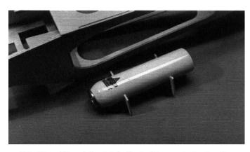
■ Mount the air tank into the holders and glue in place, using silicone calk. Then mount this air tank assembly inside the fuselage, behind Former "B" and under the fuselage top. See photo. Refer to the photo above and the photo below.
