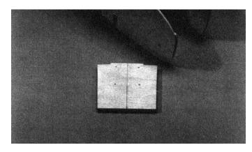
☐ When dry, mark a centerline down the middle for ease of retract mounting. This part replaces the nose spreader described in the standard kit construction.
