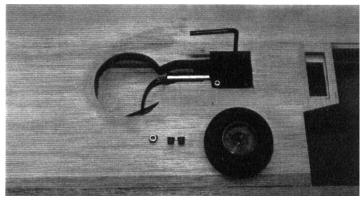
☐ Trim the length of the axle on the landing gear wires, if necessary, to fit the wheel. (The wheel shown is a 2-1/2" Robart wheel.) Follow the specific installation instructions included with your wheels.
