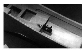
☐ Screw the retract air valve onto the air-valve holder by inserting it into the 3/8" hole.
