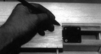
Using a 5/64 x 3 x 18" piece, mark where the retract gear will come through the sheeting.
