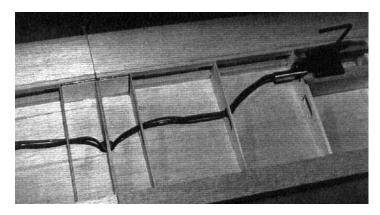
23a. After completing the L.E. and T.E. sheeting, install the air hoses through the holes in the ribs. Use the same color for each corresponding connection on each of the main gears.
