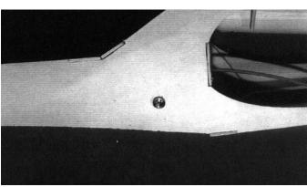
☐ Making sure you select a spot on the fuselage side which is opposite from the exhaust, and which will cause no interference with any of the servos, drill a 5/16" hole for the air fill valve.
