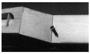
☐ Mark the center of the cabin back. Drill a 5/16" hole and mount the pressure gauge in it.
