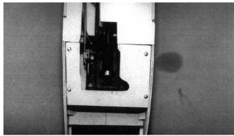
Place the retract cover on the fuse and screw down.
