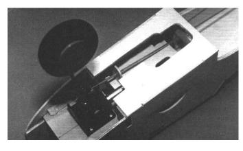
☐ Install the 1/8 x 24" tubing between the nosegear and the servo tray by threading it through the middle 1/8" hole in the air-valve holder and placing the nosegear pushrod support guide on the end closest to the nosegear.
