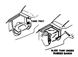
☐ Super Jet the fuel tank tray into the slots in the fuselage. Rubber band the fuel tank to the tray, making sure to insert a piece of foam between the tank and the tray.
