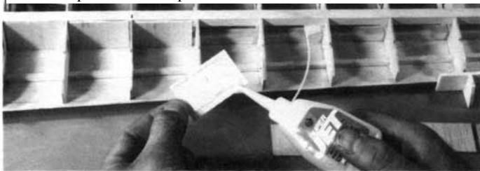
16. □□ Lay out laser-cut spar webs as shown. Glue spar webs to front of top and bottom spars.
