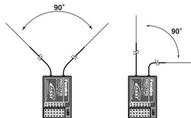
4 If your model includes metal conductive items which may impact the receiver's ability to clearly receive the radio frequency signal, we suggest mounting the receiver so that the receiver antennas exit both sides of the model. This will allow the best radio frequency signal condition at any flying attitude.
