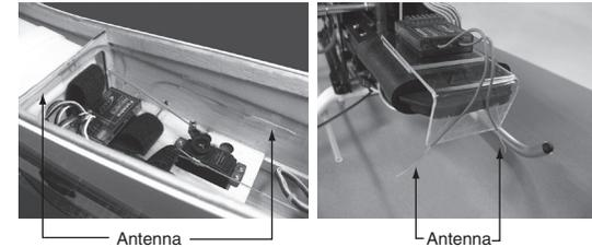
The main purpose of the photo demonstrates how the antenna should be placed. For actual installation the receiver must be wrapped with a sponge or placed with floating material to protect it from vibration.
