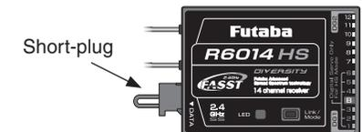
CH11 and CH12 are valid to use of MPDX-1. Other channels can not use the MPDX-1.
