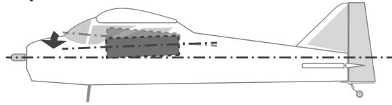
In this case, adjust so that the GYA460 is mounted slightly downward.
