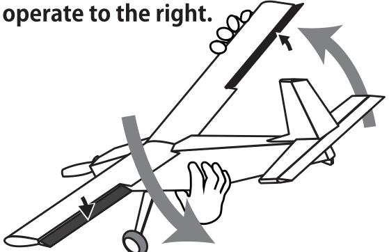
Tilt the airplane with its nose upward and check that the elevator operates downward.
