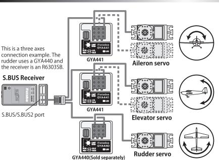
S.BUS connection makes the wiring extremely simple. The GYA440 and GYA441 can be connected by one 3-way hub. The aileron, elevator, and rudder servos are output from the gyro. Servos other than S.BUS servos can also be used. When an R6303SB is used the CH switching mode is set to group 7. The normal group 7 CH outputs are CH3, CH11, and CH12. CH3 is the throttle channel and CH11 and CH12 are spare channels.
