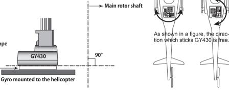
In the rudder neutral position, connect the linkage at the position at which the servo horn and control wire are perpendicular
