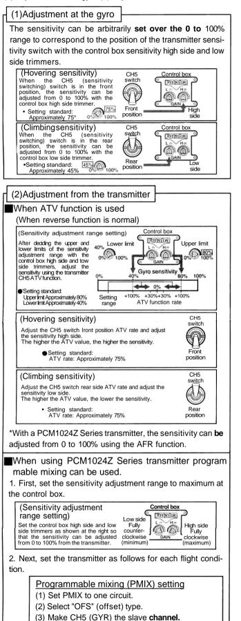
In this state, the gyro sensitivity for each flight condition (hovering, forward flight, etc.) can be arbitrarily set
