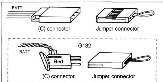
Connect the following to the (C) connector (control amplifier BATT):
