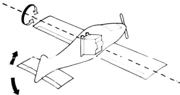
•When the gyro is mounted 180° out of phase, the direction of the correcting mix will be reversed.
