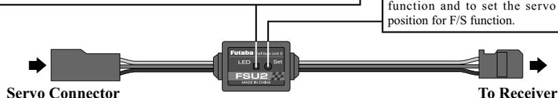
**How to check the activation voltage of B-F/S function**
