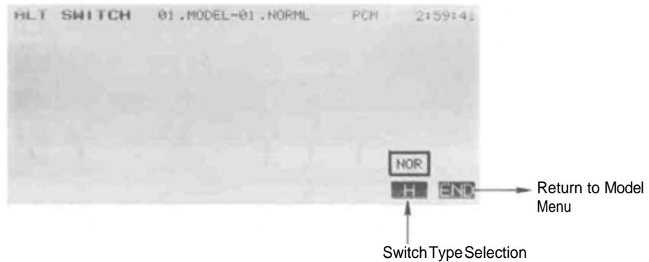
Use the H key to select the switch type. NOR = normal switch action (turns off upon release), ALT = Alternate switch action (stays on until pulled again).
