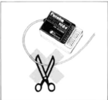
Be sure that you do not shorten the receiver antenna, either by cutting some off, or by coiling the excess up. Instead, let the excess length trail behind or below the aircraft. Cutting the antenna will reduce the effective range of the system and increase the chance of interference.
