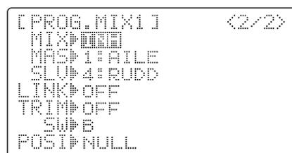
Your 9C super contains five separate linear programmable mixes (**ACRO** and **GLID. HELI** has 2). (Note that mixer #6-7's mixing **RATE**s are set with a 5-point curve. see *CURVE MIXES*, p. 63.)
