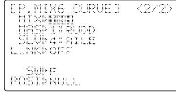
Your 9C super’s **ACRO/GLID** programs contain two separate curve programmable mixes. **HELI** contains one. There are a variety of reasons you might want curve mixes — usually where a linear mix doesn’t fit your needs along the whole range. One pre-programmed curve mix is the **THROTTLE-NEEDLE** function. This curve is adjustable at 5 points, allowing you to adjust the motor’s tuning at 5 points along its RPM range.
