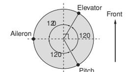
**HELI SR-3s Type:** pushrods positioned as shown. Fundamentally, the servo operations of **SR-3s** type are almost same as **SR-3** type. However, the servo arrangement about elevator operation differs.
