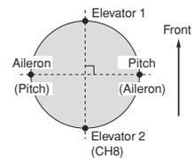
**HELI SR-3 Type:** pushrods positioned as shown. With Aileron inputs, the aileron and pitch servos tilt the swashplate left and right; with Elevator inputs, the three servos tilt the swashplate fore and aft; with Pitch inputs, all three servos raise the swashplate up and down.
