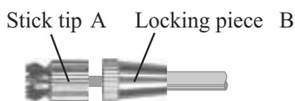
You may change the length of the control sticks to make your transmitter more comfortable to hold and operate. To lengthen or shorten your transmitter's sticks, first unlock the stick tip by holding locking piece B and turning stick tip A counterclockwise. Next, move the locking piece B up or down (to lengthen or shorten). When the length feels comfortable, lock the position by turning locking piece B counterclockwise.
