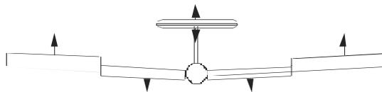
**BUTTERFLY** (often called "crow" - see **GLID**, p. 71 for details) simultaneously moves the flap, twin ailerons and elevator, and is usually used to make steep descents or to limit increases in airspeed in dives.
