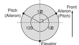
**HELI SN-3 Type:** pushrods positioned as shown. With Aileron inputs, the three servos tilt the swashplate left and right; with Elevator inputs, the elevator and pitch servos tilt the swashplate fore and aft; with Pitch inputs, all three servos raise the swashplate up and down.
