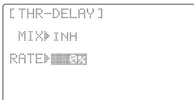
The **THROTTLE DELAY** function is used to slow the response of the throttle servo to simulate the slow response of a turbine engine. A **40%** delay setting corresponds to about a one-second delay, while a **100%** delay takes about eight seconds to respond. For helicopters, see **DELAYS**, p. 92.
