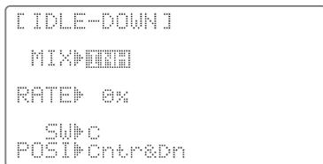
**Important note:** The **IDLE-DOWN** function is not normally used when starting the engine, and its accidental operation may keep your engine from starting. The 9C super warns that **IDLE-DOWN** is on when the transmitter is turned on. Be sure to turn off the function, or override the warning by pressing both 2 *SELECT/CURSOR* keys in unison and holding for 1 second if you intended the function to be on.
