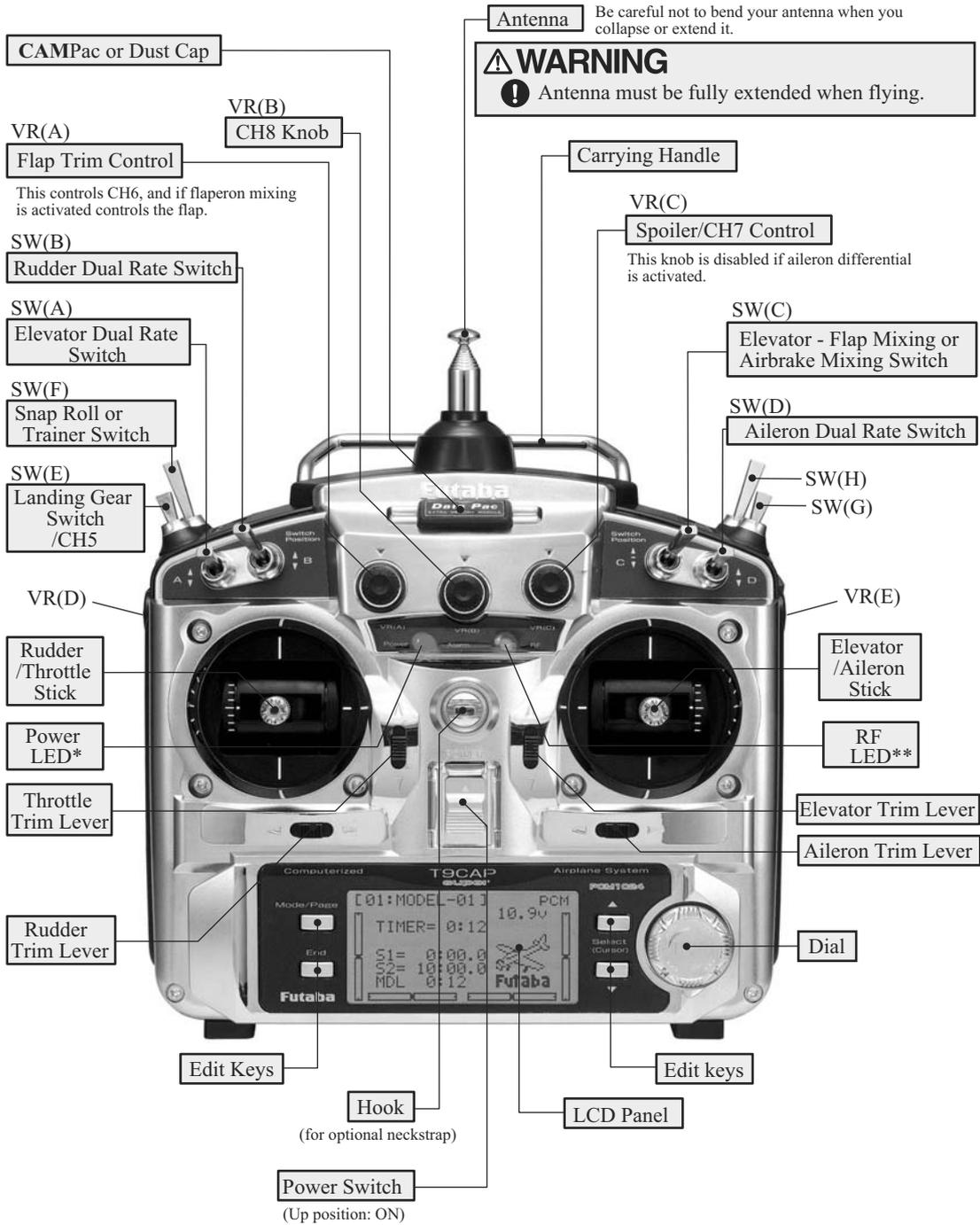
This figure shows the default switch assignments for a 9CA super Mode 2 system as supplied by the factory. You can change many of the switch positions or functions by selecting a new position within the setting menu for the function you wish to move. (Example: move aileron dual rates to switch C to create triple rates. See p. 35 for details.)
