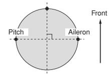
**HELI SWH4 Type:** pushrods positioned as shown. With Aileron inputs, the aileron and pitch servos tilt the swashplate left and right; with Elevator inputs, the servos tilt the swashplate fore and aft; with Pitch inputs, all four servos raise the swashplate up and down.
