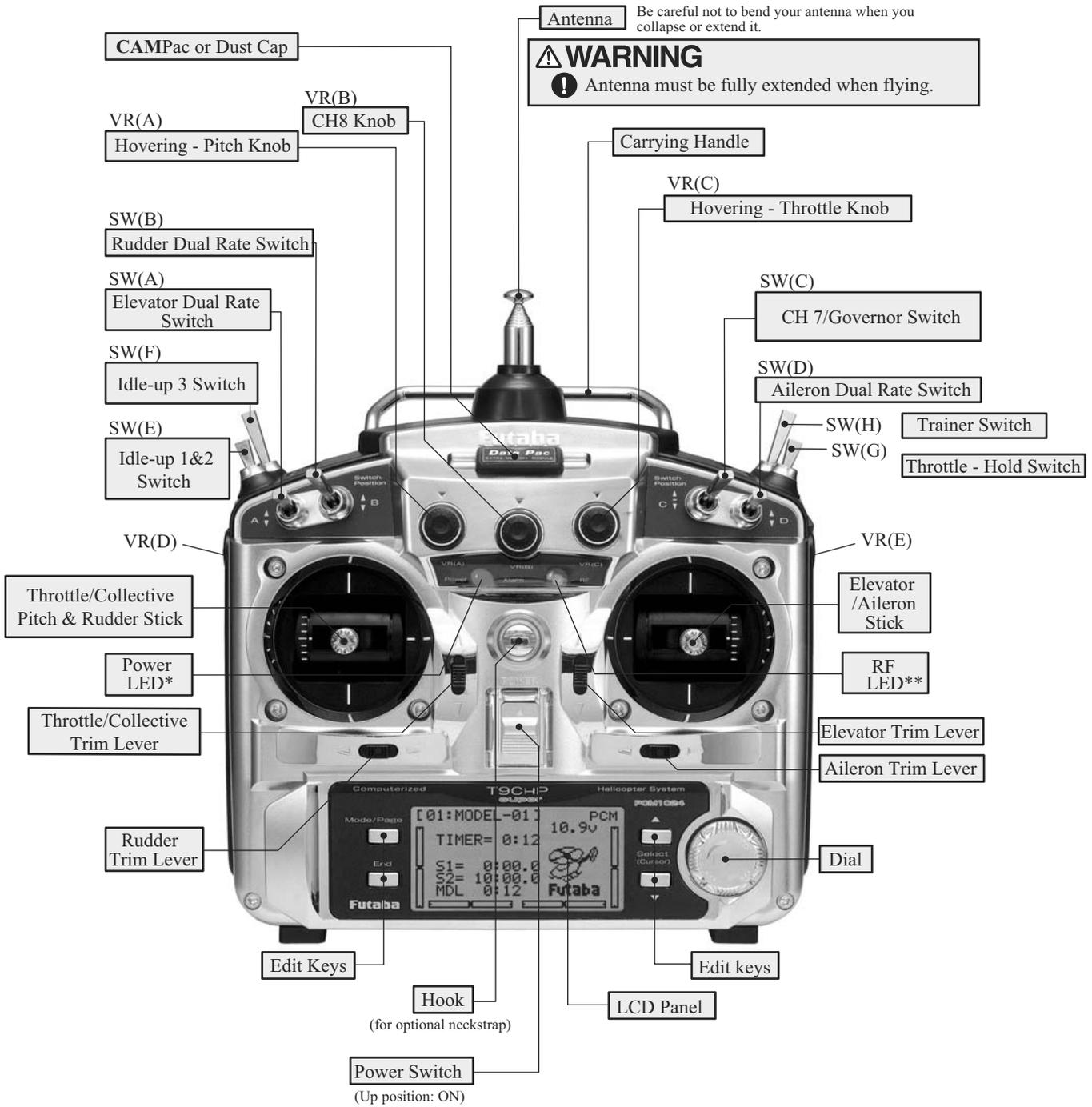
This figure shows the default switch assignments for a 9CH super Mode 2 system as supplied by the factory. You can change many of the switch positions or functions by selecting a new position within the setting menu for the function you wish to move. (Example: move aileron dual rates to switch C to create triple rates. See p. 35 for details.)
