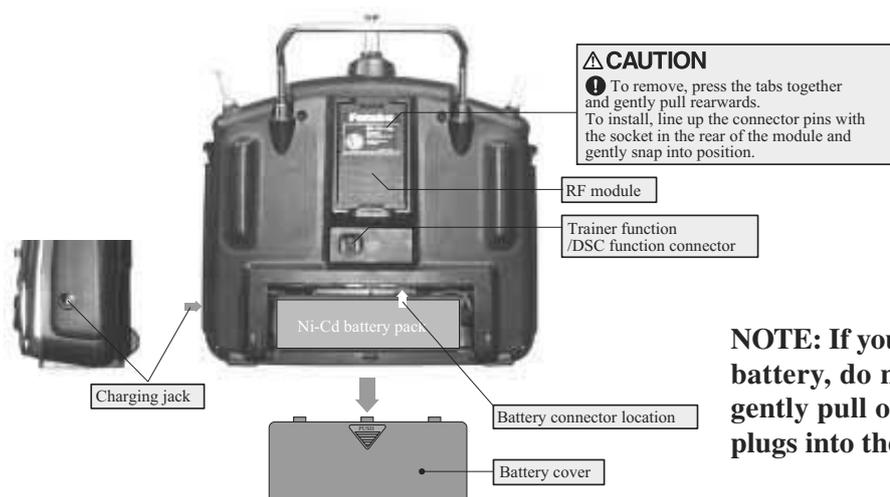
**NOTE:** If you need to remove or replace the transmitter battery, do not pull on its wires to remove it. Instead, gently pull on the connector's plastic housing where it plugs into the transmitter.
