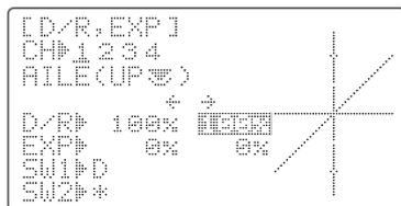
**Dual/Triple Rates:** reduce/increase the servo travel by flipping a switch, or (**ACRO/GLIDER**) they can be engaged by any stick position. Dual rates affect the control listed, such as aileron, not just a single (ex: channel 1) servo. For example, adjusting aileron dual rate will affect both aileron servos when using **FLAPERON** or **AIL-DIF**, and both aileron and elevator servos' travel when using **AILEVATOR** or **ELEVON** or a CCPM helicopter.
