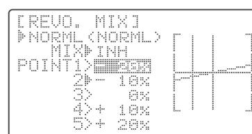
**REVO. MIX**: This 5-point curve mix adds opposite rudder input to counteract the changes in torque when the speed and collective pitch of the blades is changed.
