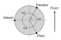
Use the reversing function (REV) as necessary to get the proper aileron, elevator, and pitch operations.
