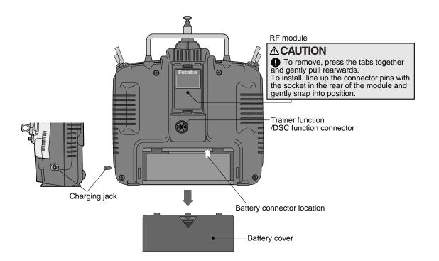
NOTE: If you need to remove or replace the transmitter battery, do not pull on its wires to remove it. Instead, gently pull on the connector's plastic housing where it plugs in to the transmitter.
