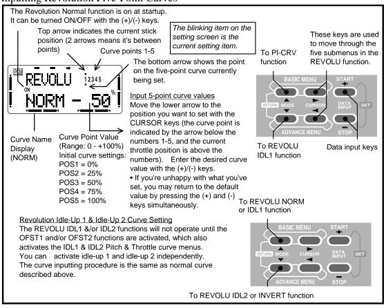
PI-CRV — Pitch Curve (Normal, Idle-Up1 & 2, Hold, Inverted)
