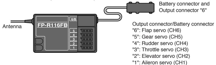
Output connector/Battery connector
