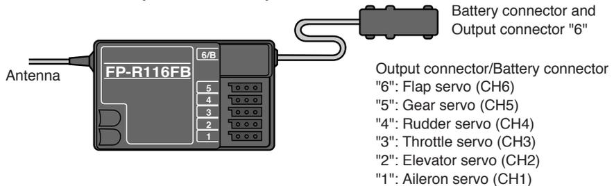
Output connector/Battery connector
