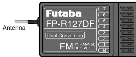
Output connector/Battery connector
