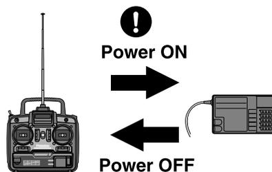
If the power switch is turned off in the opposite order, the engine may go to full throttle unexpectedly and cause an injury.
