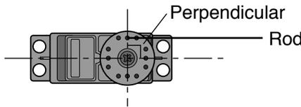
Check that when trimmed to the center, the servo horn is perpendicular to the servo and check the neutral position of the fuselage control surfaces (aileron, elevator, rudder, etc.). If the neutral position has changed, reset it by adjusting the length of the rod with the linkage rod adjuster.
