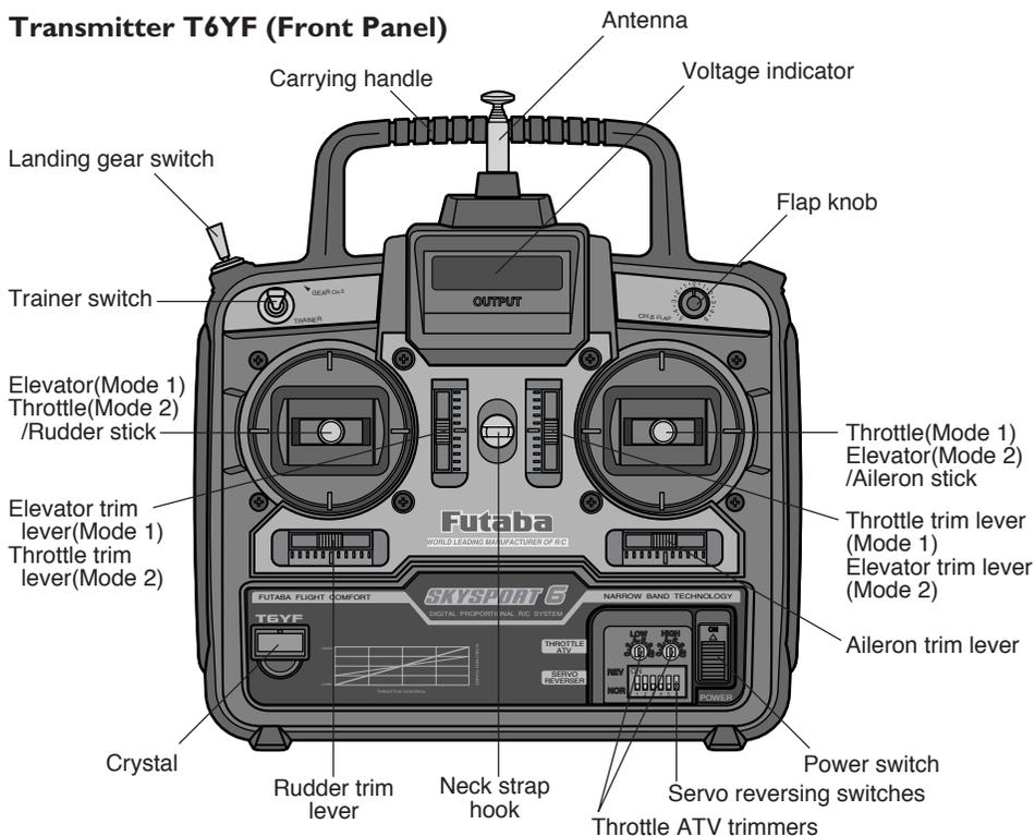
**Power switch:** Turns the transmitter on or off. In the upper position, the power is turned on.
