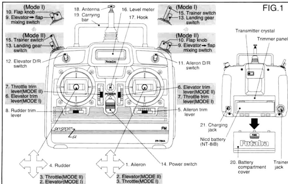
This section describes how to operate the transmitter. The numbers in the text correspond to the numbers in FIG. 1. For a definition of special terms, see "GLOSSARY OF TERMS" on page 8.
