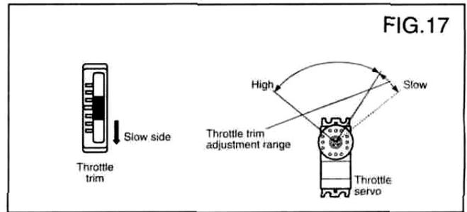
7)After connecting the linkages and checking the operating directions and amounts, start the engine and adjust the engine needle, then fly the airplane and trim the servos.
