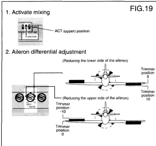
\* Applying differential by reducing the low side of the aileron: Adjust between DIFF.RATE trimmer positions 0 and 10 (right half of trimmer). At position 10, differential is not applied. At position 0 (trimmer center), the reducing amount is maximum.
