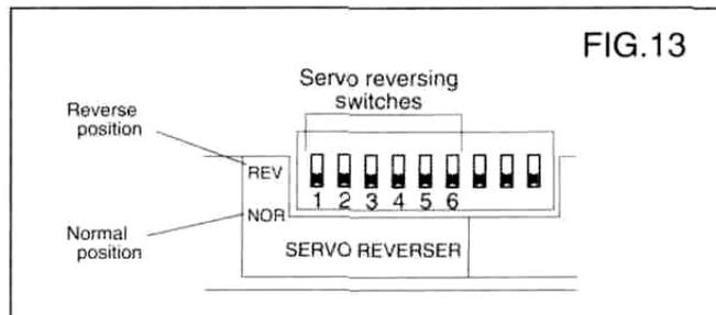
The lower (NOR) position is the normal position and the upper (REV) position is the reverse position.
