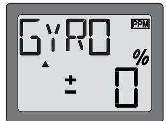
Flip the gyro (CH5) switch up and down. This will cause the arrow points up and down on the display simultaneously with switching operation and show the position of the switch. Push up or down DATA INPUT lever to set the gyro gains both switch up and down position. Gyro gain can be adjust from -100% to +100%.
