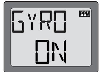
5. Push the SELECT key once. This will show the gyro gain setting and flashing **“%”** symbol on the display.
