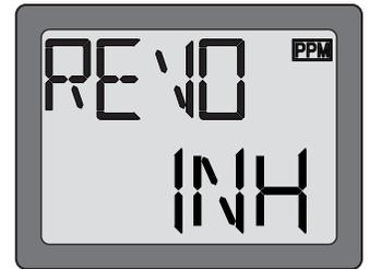
2. Push the DATA INPUT lever upward. This will cause the flashing “INH” display to change to a flashing “ON” display. Now the “REVO” function is on.
