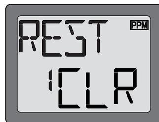
The existing modulation and swashplate type settings are not reset. If the power switch is turned off while reset is underway, the data may not be reset.
