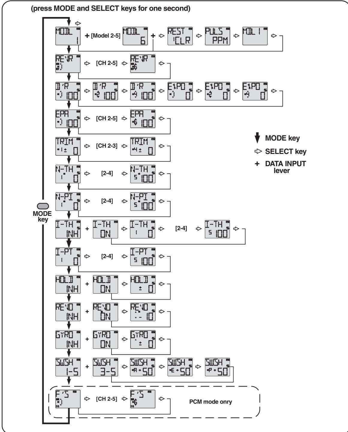
Simultaneously Press the "MODE" and "SELECT" keys and hold them down for one second to enter the programming mode. Press the keys again (or turn off the transmitter) to exit the programming mode.
