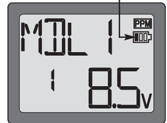
**Note:** When the transmitter voltage reads **8.9 Volts** you will still have approximately ten minutes (or less) before losing operational range, so this is the recommended **absolute minimum** voltage. If the transmitter ever reaches 8.9 Volts, land as soon as safely possible. A more reasonable margin of safety would be to quit flying for the day (or recharge the batteries) when the transmitter battery.
