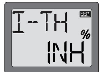
2. Push the DATA INPUT lever upward. This will cause the flashing “INH” display to change to a flashing “ON” display. Now the I-TH function is on. Push the SELECT key, throttle stick position number will appears on left side of display and “%” is blinks.
