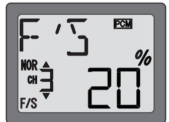
4. Verify that your failsafe programming works by switching off transmitter power and observing the motion of the servos.
