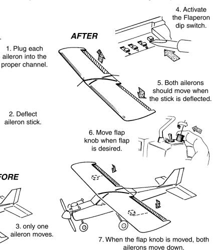
• This radio cannot support two aileron servos on separate receiver channels AND a separate flap servo at the same time. If your model requires both twin aileron servos and flaps, you must use a y-harness to drive the two aileron servos. Also note that this radio cannot support a flaperon-to-elevator mix. If you have flaperons active, the flap-to-elevator pot sets up aileron differential, not a mix.
