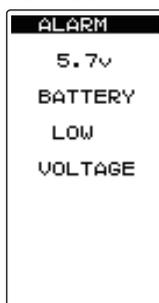
If the transmitter battery voltage drops to 4.1V (when using Futaba rechargeable type battery: 4.9V) or less, an audible alarm will sound and "BATTERY LOW VOLTAGE" will be displayed on the LCD screen.
