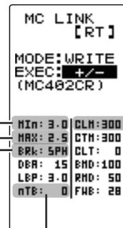
"Min" which sets the frequency when the load is small, is set to the high frequency side (large value) when extension is desired after straight-away and curves.
