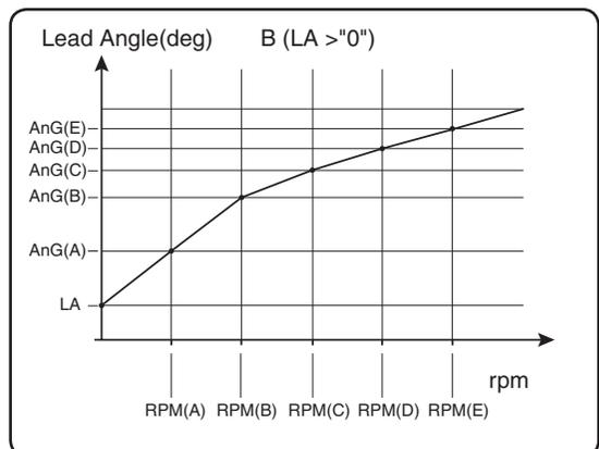
When using in races in which the lead angle setting function is inhibited by the ESC, set LAU (LEAD ANGLE USE) to OFF. The LAU setting has priority over TBM-(TURBO MODE). If LAU is set to "OFF", the lead angle setting function can be turned off even if TBM is set to "LV1" or "LV2". The MC940,960CR shows that the lead angle setting function is OFF ("0" timing) by flashing an LED.
