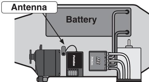
Install the receiver as far away as possible from the battery, motor controller, motor, silicon cord and other noise sources. Keep it away from the antenna wire, in particular.
