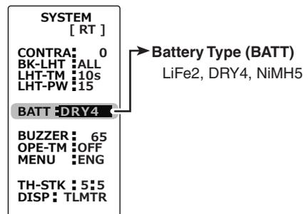
**Note:** If used with the incorrect setting, a normal low battery alarm will not be generated and the system may stop before the battery alarm is generated. The usage time may also become extremely short.
