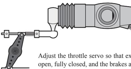
Adjust the throttle servo so that excessive force is not applied when the engine carburetor is fully open, fully closed, and the brakes are applied fully.
