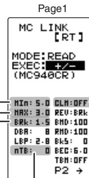
"Min" which sets the frequency when the load is small, is set to the high frequency side (large value) when extension is desired after straight-aways and curves.
