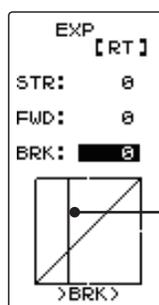
Vertical cursor moves in step with throttle stick operation.
