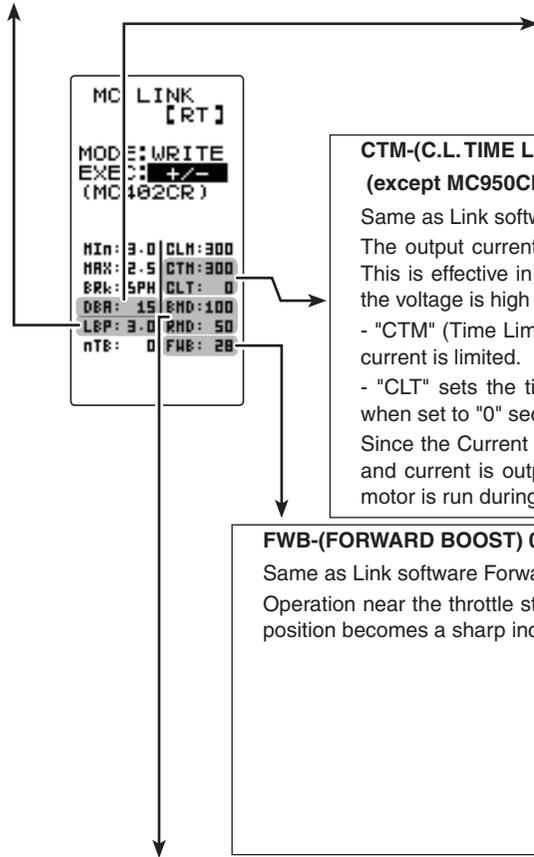
**CTM-(C.L. TIME LIMIT) 50A~300A /CLT-(C.L. TIMER) 0sec(OFF)~240sec (except MC950CR)**
