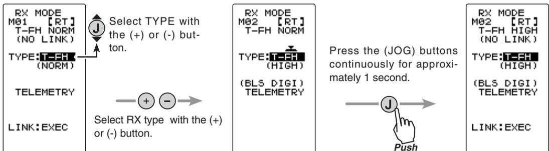
\*When using an FHSS (R603GF/R2004F, etc.) or S-FHSS(SFH) system (R2104GF, R204GF-E, etc.) receiver, after the end of setting up to here set the transmitter power switch to OFF and go to **"Receivers other than T-FHSS"** .
