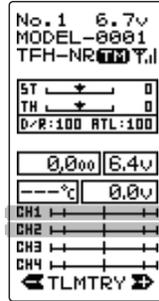
→ Servo operation of steering channel (CH1) can be checked.
