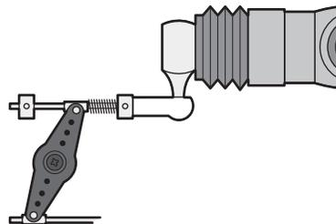
Adjust the throttle servo so that excessive force is not applied when the engine carburetor is fully open, fully closed, and the brakes are applied fully.
