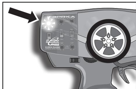
The low battery alarm is meant to be a safety feature only. Do NOT operate your radio below low battery. Always shut your radio off as soon as possible after the low battery warning loss of control.
