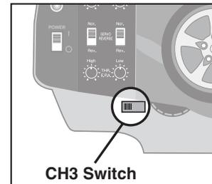
CH3 cannot operate EPA function and servo linearly.
