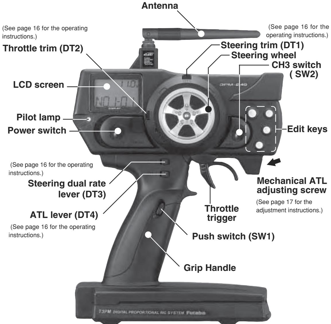
\*The switches and levers in the figure are shown in the initial setting position.
