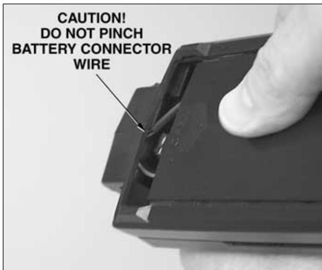
**⚠ CAUTION - DO NOT** pinch the NiCd battery wire when sliding the lid closed. If the wire is damaged, abnormal heating and fire may result.
