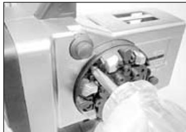
5. Remove the 4 screws from the wheel unit.
