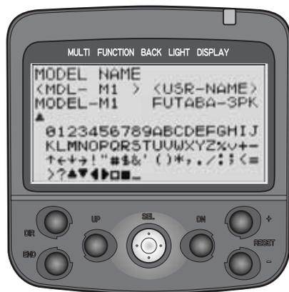
**DEFINITION:** Provides a 10-character name for each of the model memories in the transmitter to easily select the correct setup for the model currently in use. Also provides a 10-character user name that is constant to all model memories.
