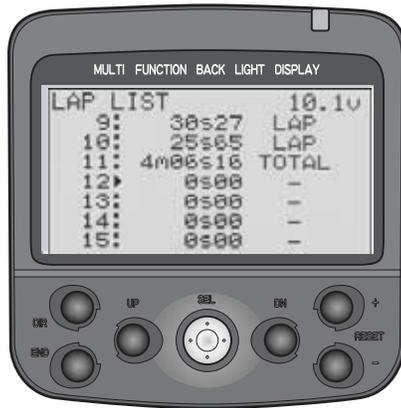
**DEFINITION:** Displays all stored lap times, up to 100, and also stores total race time, including run time after last but before reset/stop.
