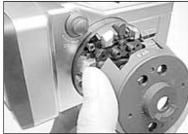
4. Remove the wheel unit cover. Be very careful or the wheel shaft will fall out.
