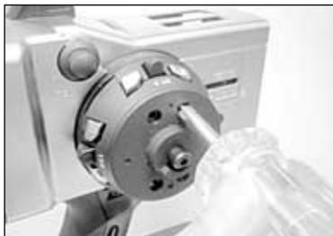
3. Remove the 4 screws from the wheel unit cover.
