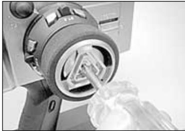
1. After removing the wheel cap, carefully remove the screw holding the steering wheel.
