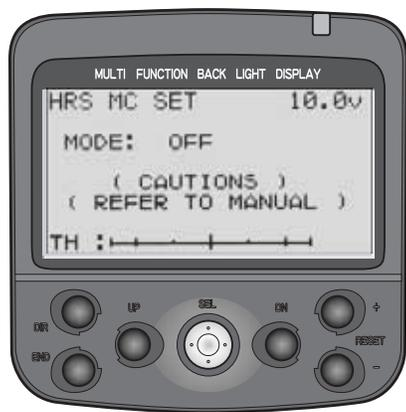
**DEFINITION:** Adjusts frame rate of transmitter output to throttle channel for setting up non-Futaba ESCs with HRS systems. HRS frame rate is faster than many speed controls can properly read to complete their auto setups.
