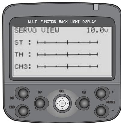
**DEFINITION:** Shows the exact outputs the transmitter is sending to the servos. Allows for easy testing/experimenting even when receiver and servos are not yet installed.
