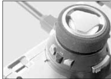
1. Remove the wheel back cover using 2.5mm hex wrench.
