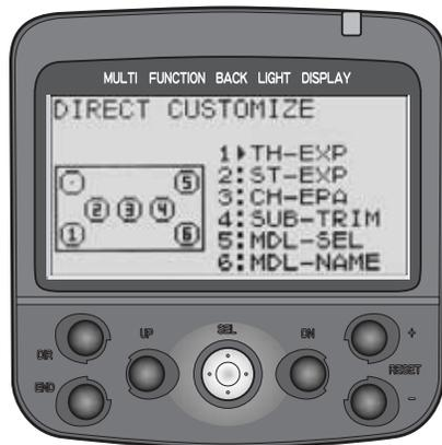
**DEFINITION:** Customize what functions are available at the push of 2 buttons (Direct menu and one more) by adjusting the Direct Selection menu. Note that direct menu selection/exit is always the DIR button.
