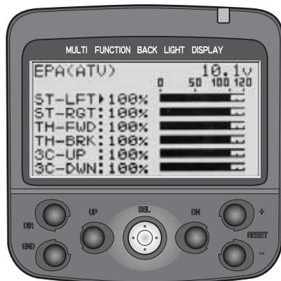
**DEFINITION:** End point, commonly called EPA or ATV, adjusts (shortens or lengthens) the total travel of the servo. For example, a steering servo travels 60° each way. Decreasing the right EPA to 50% results in a steering servo that will move 60° to the left but only 30° to the right.
