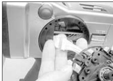
6. Disconnect the wheel unit wiring harness.
