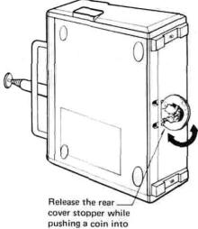
• Remove the rear cover of the transmitter **as** shown in Fig. 4 and load the 7 pen-cell batteries in the correct polarity.
