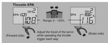
Be sure that your throttle linkage does not apply excessive force to the servo.
