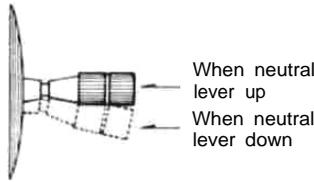
If the neutral lever is moved, the neutral position of the stick lever can be adjusted in two steps as shown in the figure.
