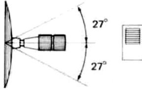
When the neutral lever is up, the throttle stick can be adjusted to a total of 54°, 27° up and 27° down, from the neutral position. This position is best for electric cars and other models with which the center of the speed controller is the neutral position.
