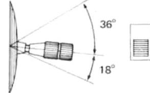
When the neutral lever is down, the throttle stick can be adjusted to a total of 54°, 36° up and 18° down (2-to-1), from the neutral position. This position is best for engine-drive cars or other models with which the speed controller neutral position is offset.
