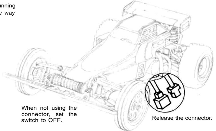
When not using the connector, set the switch to OFF.
