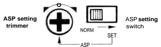
3. Then complete adjustment by setting the ASP setting switch to the NORM side. (If the switch is not switched to the NORM side, the throttle servo will not be controlled by the throttle stick.)
