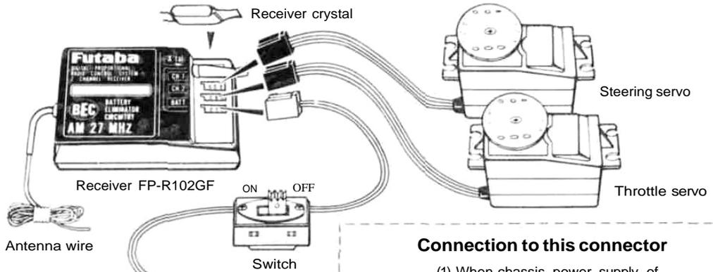
Connect the servo and switch as shown in the figure and extend the transmitter and receiver antenna fully.
