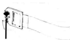
The flag can be attached to and removed from the **end** of the antenna with one **touch**.
