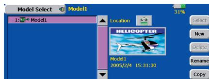
This is convenient when calling a model after registering the model names in advance. (The data of up to 30 models can be saved at the transmitter. Data can also be saved to the accessory Data-Pack.)
