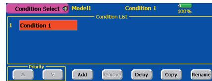
\*When a new condition is added, "Condition1" data is automatically copied.
