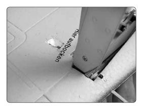
10. Using the punch, gently push the hinge pin out of the hinge and into the exit area created on steps 4-7. Using pliers, remove the brass hinge pin.
