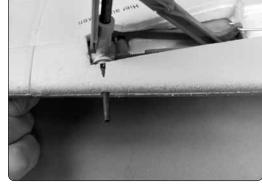
the 3x30mm carbon fiber tube into the hole made at the leading edge. Apply foam safe CA to the area around the carbon fiber tube.
