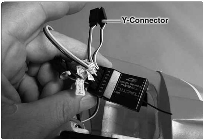
2. Connect the elevator, ESC (throttle) and rudder servo wires to the corresponding receptacles in the receiver—each is labeled Ch. 2, 3 & 4 accordingly. Connect the included Y-connector into channel 1 (ailerons) and connect the flap and light wires to available auxiliary receptacles in the receiver.
