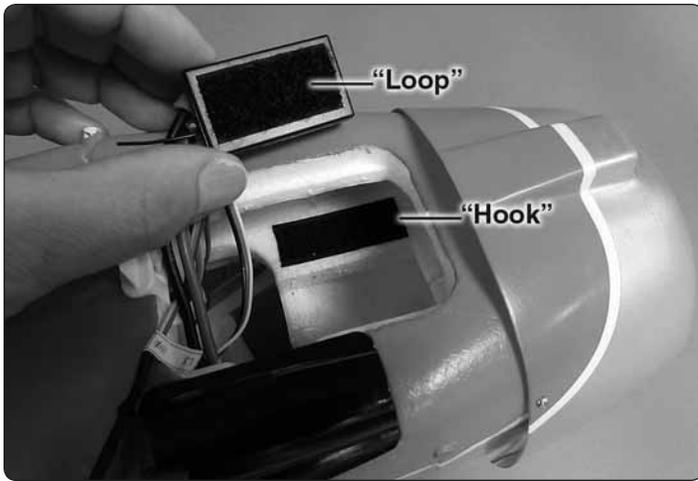
1. Apply a strip of the softer, "loop" side of the included double-sided adhesive-back Velcro® strip to your receiver (not included) and a strip of the rougher, "hook" side inside the fuselage where shown.
