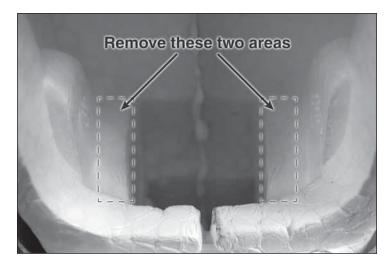
1. Use a #11 blade to cut and remove the excess material from each side of the fuselage.
