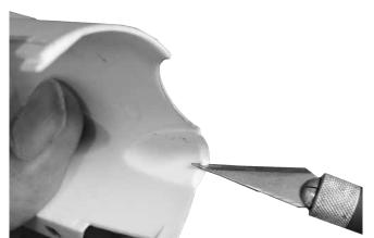
If you notice the motor wires catching on the inlet shroud on the back of the turtledeck, remove the turtledeck and use a hobby knife to chamfer the inside of the shroud to accommodate the wires.
