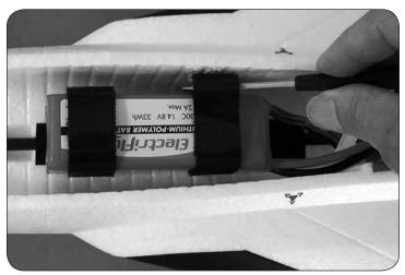
When removing the battery, the hook and loop material is easily separated with a screwdriver.
