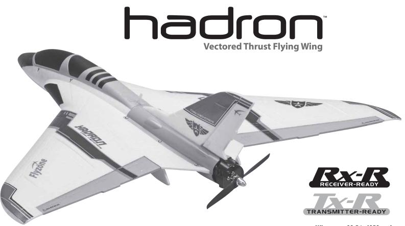
Wingspan: 33.5 in [850mm] Wing Area: 408 sq in [26.3 dm<sup>2</sup>] Weight: 29.6 – 31.3 oz [840 – 885 g] Wing Loading: 10.4 – 11.0 oz/sq ft [32 – 34 g/dm<sup>2</sup>] Length: 33.5 in [850mm] Radio: 6-channel computer radio with elevon mixing Motor: 35-36-2200kV Outrunner, 40A ESC
