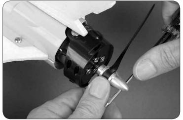
2. Fit the propeller to the collet assembly in the "tractor" configuration (front of the prop facing forward) and tighten the nut using a screwdriver shaft to torque it down.
