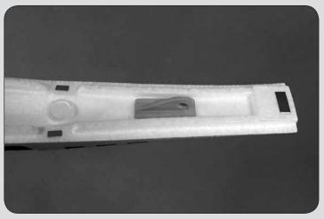
2. Use medium-grit sandpaper to roughen the inside of the canopy where the hook is to be glued. Use CA to securely glue the base into position where shown.
