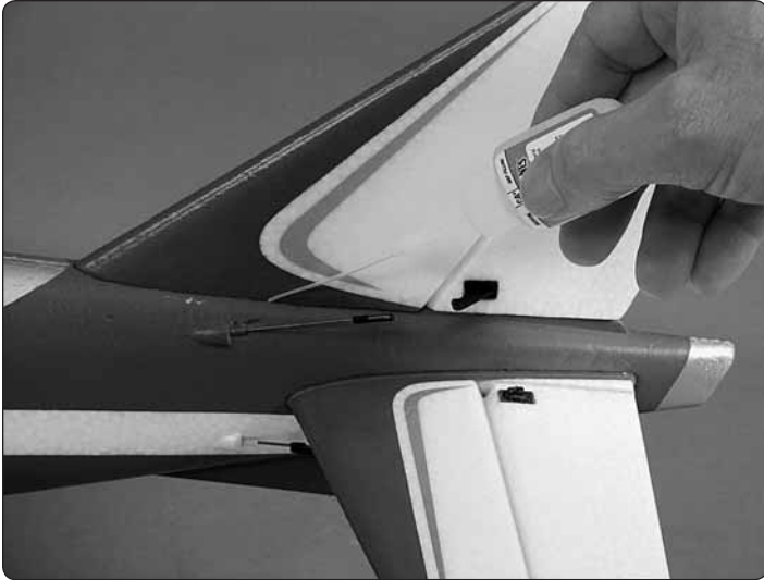
❑ 6. Apply medium or thin CA all the way around the stab and fin to glue them to the fuselage.
