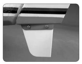
2. Install two 2x4mm Phillips head machine screws through the predrilled holes in the water rudder and groove.
