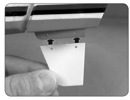
1. Place the water rudder in the groove on the lower portion of the rudder as shown.
