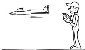
Adjust the elevator and rudder trims so the plane flies straight and horizontal when the sticks are free.
