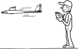
Adjust the elevator and rudder trims so the plane flies straight and horizontal when the sticks are free.
