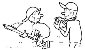
4. In case the motor starts rotating accidentally, have an assistant hold the rear part of the plane securely.
