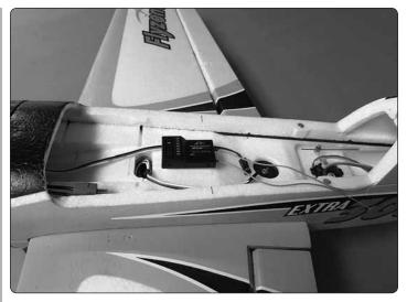
□ 9. Mount your receiver in the fuselage with the included short, adhesive-back hook-and-loop strip—note that the *high end* of the receiver (that has the servo plugs sticking out) must be *ahead* of the instrument panel in the canopy hatch (marked by a line in the photo approximately 2-1/2" [65mm] ahead of the wing bolt).
