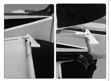
□ 4. Fit the elevator and rudder pushrods into the *middle* hole in their respective control horns and secure with the **90° pushrod keepers**.
