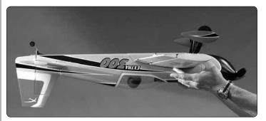
□ 4. With the model in ready-to-fly condition and the battery and propeller installed, lift the model by the wing with your fingertips between the balance range. As long as the Extra balances anywhere within the range the C.G. is okay. If the model doesn't balance, move the battery forward or aft until you can get it to balance.
