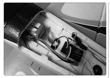
□ 5. Mark the location in the fuselage where to position the battery to balance. Remove the pins if you used them.
