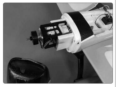
□ 1. Temporarily pop the cowl off the fuselage just to see how the motor and ESC are mounted and to make sure everything is connected properly. Reinstall the cowl.
