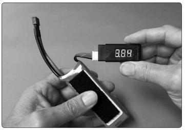
Additionally, or if you don't have a charger with a digital readout to find out how much capacity you used during a flight, use a LiPo cell checker to check individual cell voltage after each flight. The resting, non-loaded, individual cell voltage after a flight should be no less than **3.7 V/cell**.
