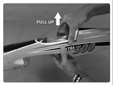
To remove the canopy hatch, grasp the base around the bottom and pull up to disengage the magnets.
