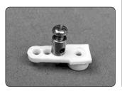
□ 5. Re-install the plastic keeper by pressing it on the pushrod screw lock connector pin. If the plastic keeper is loose and will not stay on, a new pushrod screw lock connector can be obtained by contacting *Hobbico Product Support*. The contact information is shown on page 4 of the Sensei instruction manual.
