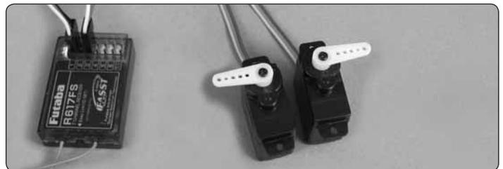
□ 1. Temporarily connect the aileron servos and ESC to your receiver and turn on your transmitter. Making sure the trims on your transmitter are centered, connect the battery to the ESC. If necessary, remove and re-mount the servo arms so they will be perpendicular as shown. Be certain to replace the servo arm screws.
