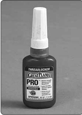
Non-permanent threadlocker should be used on all screws that thread into metal such as the motor mount screws, the set screws in the propeller hub and the screws that secure the spinner—a large amount of threadlocker is not required—just enough to “wet” the first few threads.
