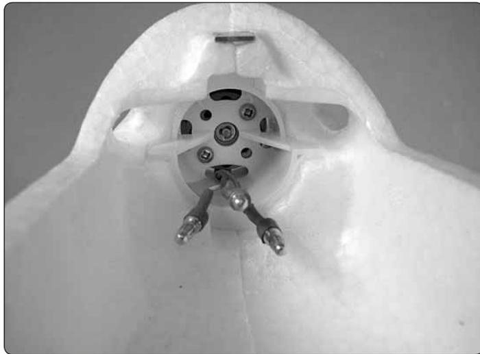
❑ 1. Guide the motor wires through the oval hole in the bottom of the motor mount. Then, mount the motor with the two 3 x 5mm screws (don't forget to use threadlocker on the screws).
