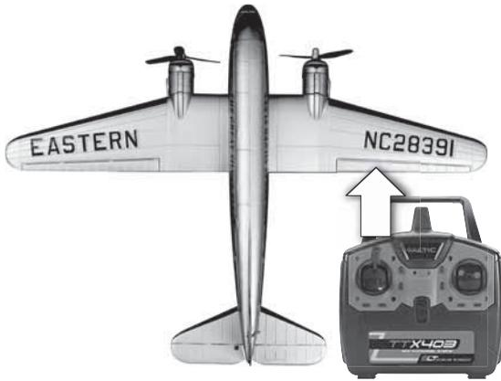
2. While holding the model by the tail, raise the throttle control stick to the maximum or high position. Hear a «Beep» sound.
