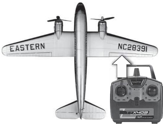
2. While holding the model by the tail, raise the throttle control stick to the maximum or high position. Hear a «Beep» sound.
