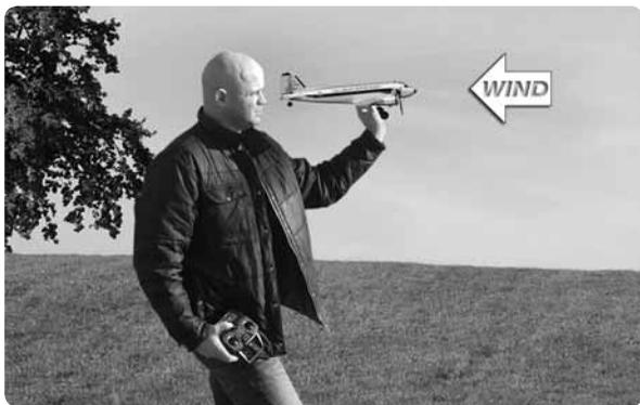
Take off (or hand launch) heading directly into the wind.
