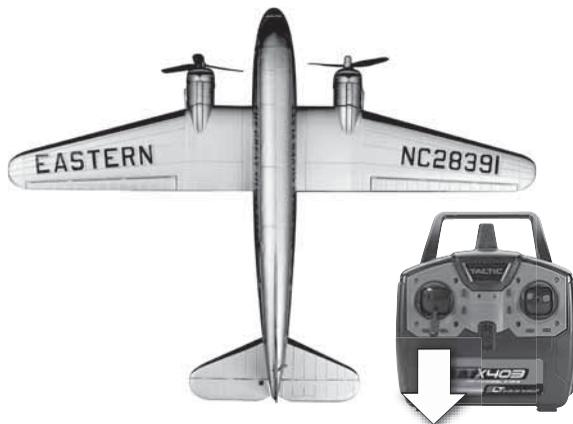
1. Switch on the transmitter and position the throttle control stick in the low or minimum position. Plug the battery into plane.
