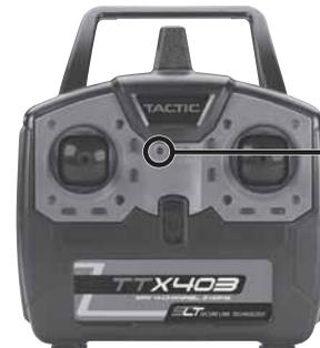
Illuminated green light indicates charging. (It may be necessary to cycle the on/off switch to begin charging.) When the LED goes out, charging is complete.
