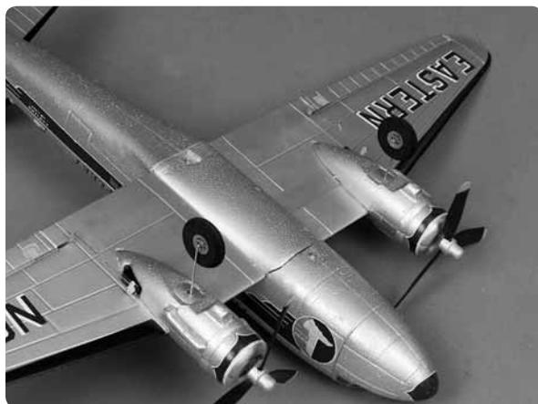
4. Insert the main landing gear. **NOTE:** The strut goes to the front of the slot.
