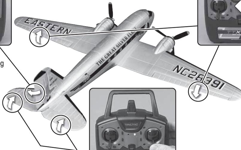
Right stick moves down, elevator moves up causing the aircraft's nose to pitch up.
