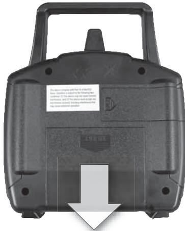
Push and slide to remove the battery door.
