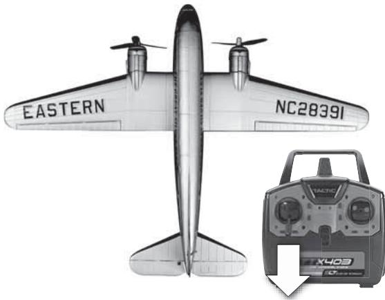
3. Return the throttle control stick to the minimum position. Hear «Beep Beep» sound. The motors are now armed and the propellers will operate if the throttle stick is raised.
