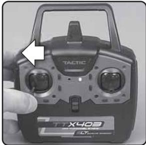
Left stick moves left, rudder moves left, causing the aircraft to yaw left. Tailwheel points right.
