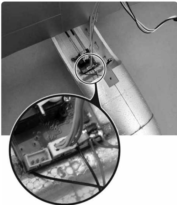
1. Plug the white micro connector from the aileron servos on the wing into the receiver board. Be careful to plug the connector in correctly.
