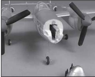
Press battery into place to secure.
