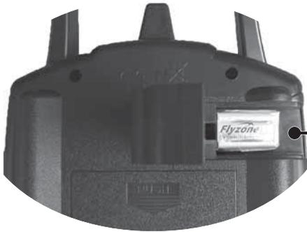
Insert battery to charge. Make sure the battery plug is oriented properly before inserting.
