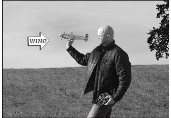
Once in the air, gain altitude to allow yourself sufficient reaction time to make a correction during flight. Once you're comfortable, adjust the aileron and elevator trims one click at a time so that the Micro P-38 Lightning flies straight and level with the control sticks centered.
