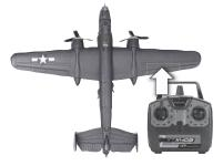
Raise the throttle control stick to the maximum or high position. Hear a «Beep» sound.
