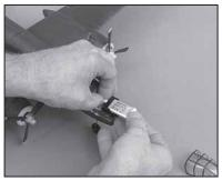
Remove nose cone. Use two fingers to secure connector during battery installation and removal.
