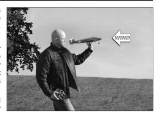
Once in the air, gain altitude to allow yourself sufficient reaction time to make a correction during flight. Once you're comfortable, adjust the aileron and elevator trims one click at a time so that the Micro B-25 Mitchell flies straight and level with the control sticks centered.
