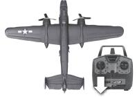
Return the throttle control stick to the minimum position. Hear «Beep Beep» sound. The motors are now armed and the propellers will operate if the throttle stick is raised.
