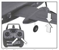
Before flight, center aileron control surface with aileron trim adjustment.
