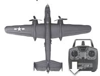
Switch on the transmitter and position the throttle control stick in the low or minimum position. Plug the battery into plane.
