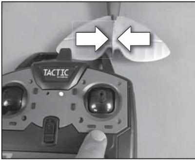
Before flight, center rudder control surface with rudder trim adjustment.
