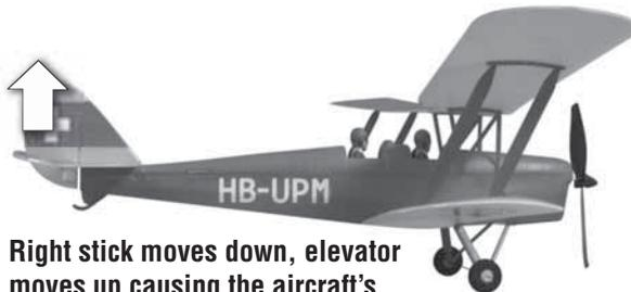
Right stick moves down, elevator moves up causing the aircraft's nose to pitch up, gaining altitude.
