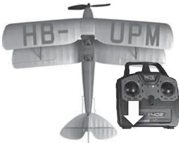
Throttle control stick is in the low or minimum position.
