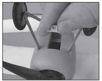
Use two fingers to secure connector during battery installation and removal.
