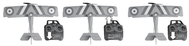
Throttle control stick is in the low or minimum position.
