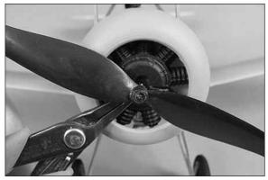
To replace or reinstall the propeller, unpower the model, then hold the motor shaft with needlenose pliers and push the propeller back onto the shaft. Once re-installed, add a drop of CA glue to the propeller to hold it to the shaft.
